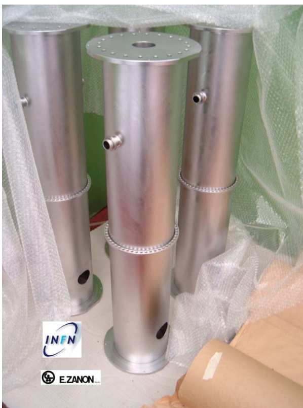
Figure 1: The low- \beta cavities under construction
