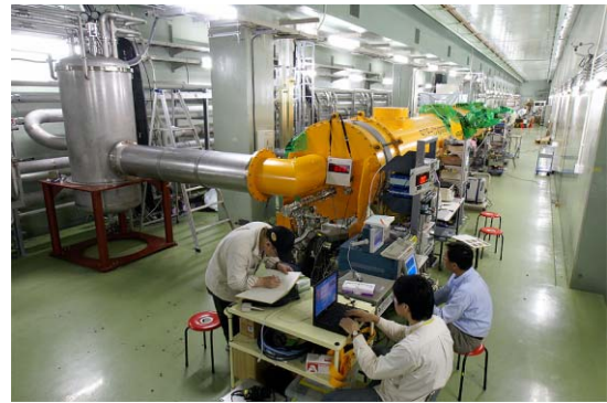
Figure 18: STF cryomodule connected with a cold valve box for the first cool-down test in the tunnel.
