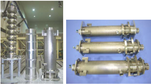
Figure 16: Before and after TIG welding of a He jacket. A magnetic shield (centre in left) was inserted in a He jacket.
