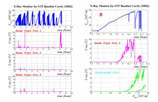
Figure 11: X-ray monitoring and scattered plot.
