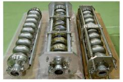
Figure 1: The STF Baseline 9-cell Cavity.
