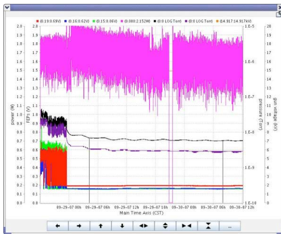
Figure 5: Processing away electron emitters with high-power pulsed RF. The blue/green/red traces are coupler electron pickup signals, the purple/black traces are coupler pressure readings, and the pink trace is the cavity transmitted power. Note how the electron signals disappear and the pressure abruptly settles after a few hours on this plot.
