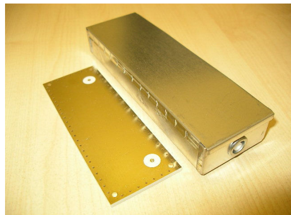
Fig. 3: Filter PCB and package
