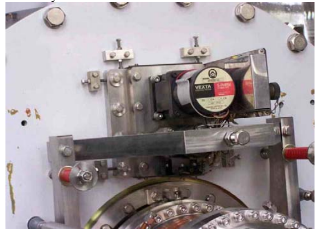
Figure 3: Mount a pair of compensation springs (red) on the tuner arm.
