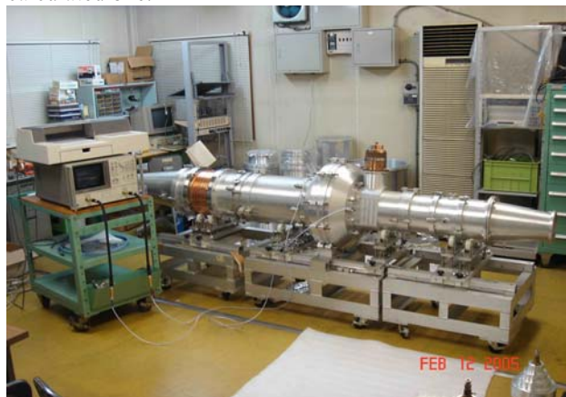
Figure 1: Aluminium model cavity in a test room.
