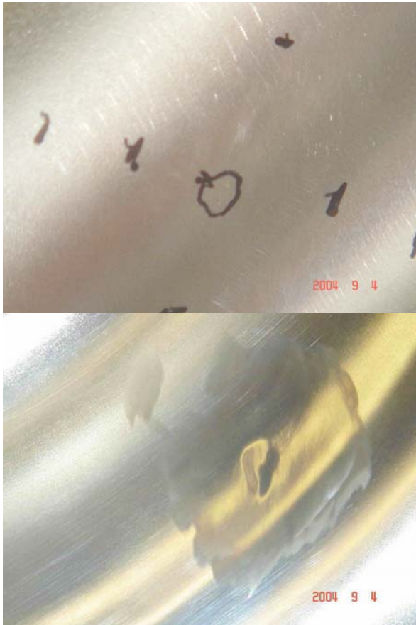
Figure 2: Before and after the mechanical local grinding.
