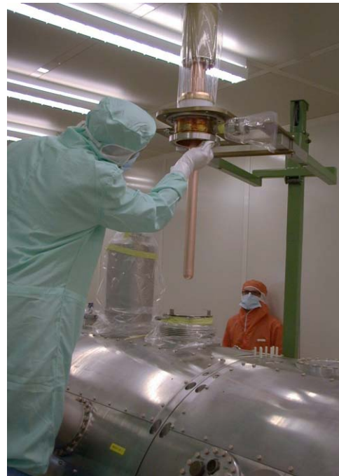
Figure 1: Coupler mounting in class 10 clean room.
