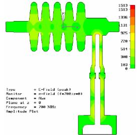
Figure 4: A standing-wave electric field distribution in the PEFP FPC with a low-beta cavity.
