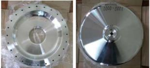
Figure 7: A female die and a male die for the central cells of the PEFP Low-beta cavity.
