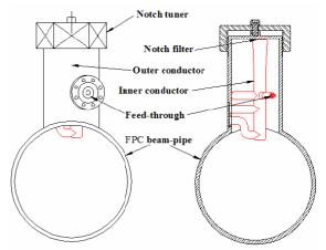
Figure 3: PEFP HOM coupler and cross-section on the FPC beam-pipe.
