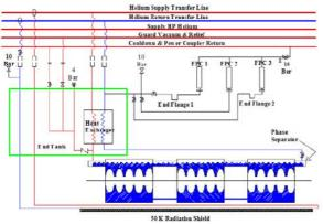
Figure 5: Cryogenic circulation schematic of the PEFP Low beat cryomodule. The blue colour means the supply coolant or cold helium liquid; and the red colour means the return coolant.
