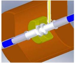
Fig.1. A schematic of the 2.85 GHz SRF cavity with a high RF power input coupler and HOM absorber
