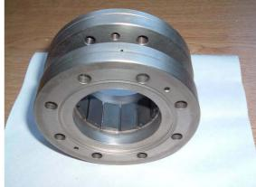
Fig 6. Ferrite HOM absorber at MIT-Bates
