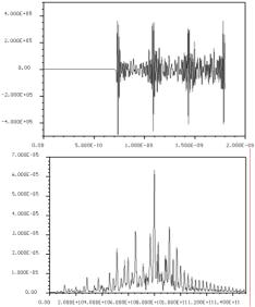
Fig 5. Examples: RF electric field at point 1 & frequency spectrum induced by 6 bunches
