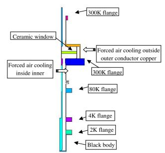
Fig 8. Thermal model for tapered coax coupler
