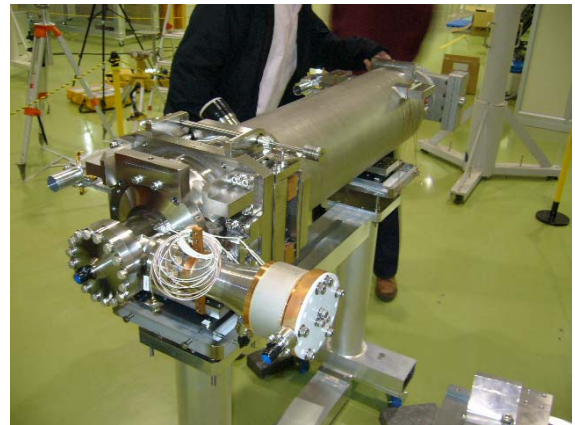
Figure 5: The STF cavity with jacket, tuner and input coupler at KEK.
