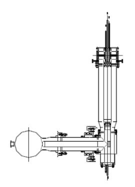
Figure 1: Schematic view of the RF input coupler
