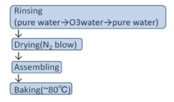
Figure 4: Prorocedure of The input coupler preparation.
