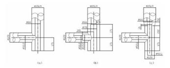
Figure 2: Schematic view of the candidates of the T-stub structures.(a)The simplest shape.(b)The diameters of inner conductor are changed at two points. (c)The diameter of inner conductor is changed using a taper.
