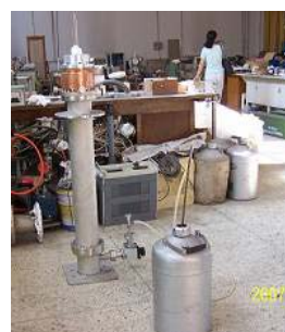
Fig9. The window and antenna stored in a special container filled with nitrogen
