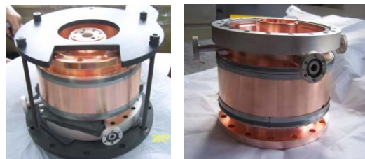
Fig5. The whole window brazing: before brazing (left) and after brazing (right)
