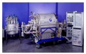
Figure 3: Cornell type module with valve box and LLRF
