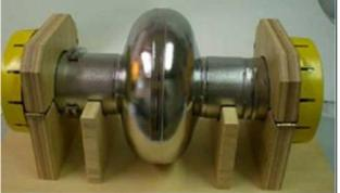
Figure 1: 1.3 GHz single crystal cavity for DESY
