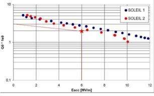
Figure 5: SOLEIL cavity test results
