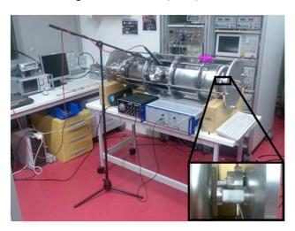
Figure 8: Setup for microphonics measurements at room temperature. The actuating piezo is installed between an endplate of the outer corset and the cavity near the beam pipe.
