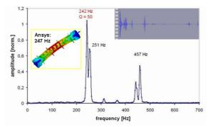
Figure 9: Measured resonances between 200 and 500 Hz. A graphic data output of an ANSYS simulation shows the displacements encoded in colours of the basic transverse mode between fixed ends measured at 242 Hz. The simulated value is 247 Hz. The recoded wave data during sweeping are displayed on top right of the graph.
