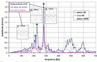
Figure 13: Microphonics at cryogenic temperatures and the impact on the rf-resonance. Three resonances are pointed out, corresponding oscilloscope pictures are shown. Case 2 at 226 Hz can clearly be detected by the piezo sensor, but has no impact on the VCO signal.
