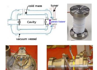
Figure 4: Scheme of the cryostat with tuner positioning on top right, a piezo from Physical Instruments (PI) top left, the mechanical tuner bottom left and beam pipe were piezo tuner shown in fig. 5 will be included close to the cooling loop in the middle (dotted line).
