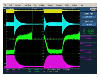
Figure 7: The VCO signal (green) as a direct indication of Lorentz-force detuning. Rf-pulse (yellow), Reflected power (blue), transmitted power (pink).
