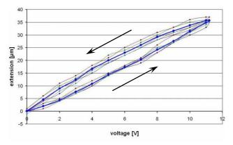
Figure 6: Measured piezo stroke hysteresis curve vs. control voltage at room temperature; slim lines for 5 individual piezos, averaging in fat blue.
