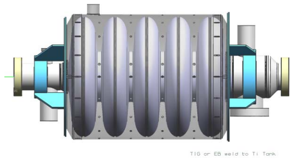
Figure 7: The shield around the cavity.
