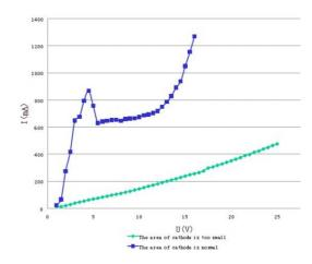
Fig 8. I-V curves with different cathode areas, the blue curve is normal. Much small area of cathode let the green curve like a line
