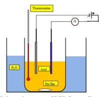
Fig.1. Schematic set-up of BEP for small samples
