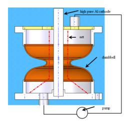
Fig3 Schematic device of BEP for dumbbell
