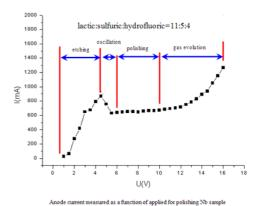
Fig. 4 Current density measured as a function of applied voltage for the polishing system
