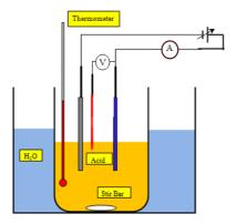
Fig.2. Schematic experiment of study Jacquet layers
