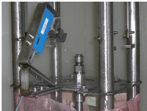
Figure 1. DESY setup for HPR water jet characterization with load-cell. The nozzle is 60° inclined with respect to the axis. For these measurements, the load cell (blue box on the left corner) has been installed parallel to the nozzle exit.
