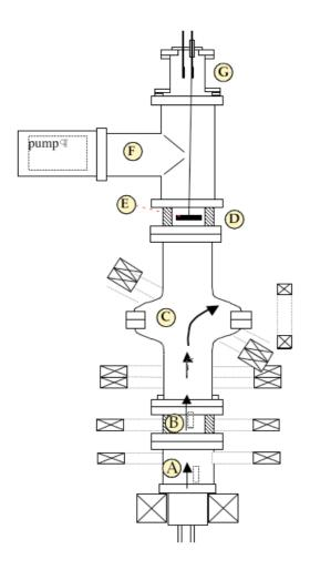
Figure 2 Magnetic configuration for cavity coating. The uppermost coil can rotate around the cavity axis to produce a uniform coating in the upper cell.
