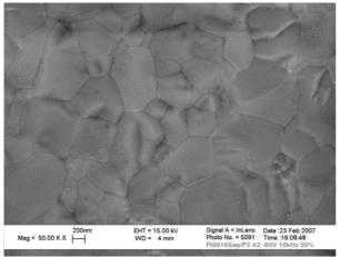
Figure 1 FEG-SEM image of a Nb film deposited on a sapphire substrate using the pulsed bias.
