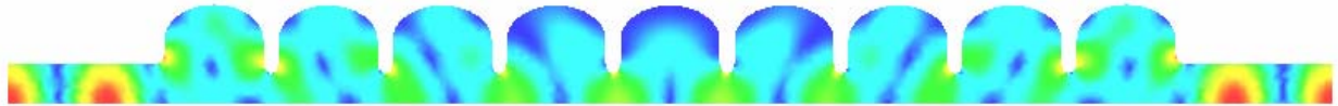
Figure 6: Analyst field plot of |E| for multi-cavity mode in the 3 rd dipole region at a frequency of 2.64203 GHz
