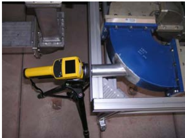
Fig.13: IR-camera to measure the surface temperature on the waveguide window during operation.
