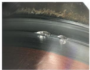
Figure 8: Damaged CF100 flange knife edge.
