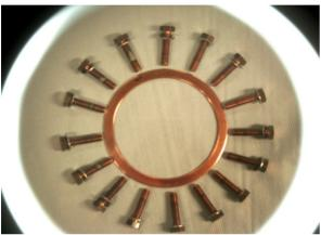
Figure 10: RF discharge stained CF100 flange screws.
