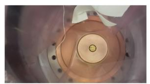
Figure 6: Cold antenna after grinding and cleaning.
