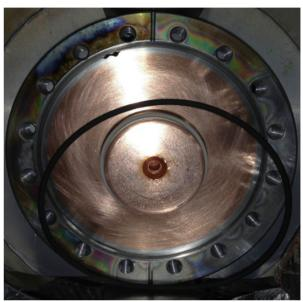
Figure 7: Forgotten O-ring on top of copper gasket.
