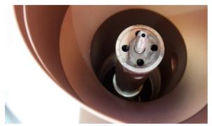
Figure 5: Burnt inner conductor of the warm part.
