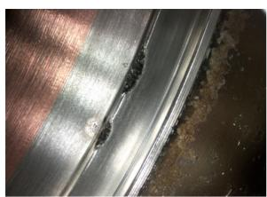
Figure 9: Burnt CF100 flange knife edge.
