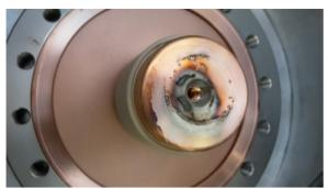
Figure 4: Burnt contact of the cold antenna.
