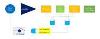
Figure 9: Overall interlock logic loop.
