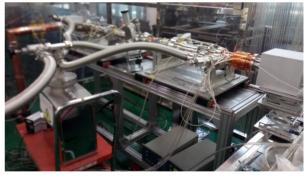
Figure 11: Setup of high power condition test stand.
