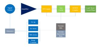
Figure 6: Logic loop of the auto-conditioning mode.
