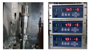
Figure 7: Vacuum gauge sensor (left) and ULVAC vacuuum gauge (right).
