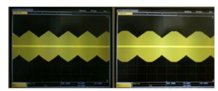
Figure 5: RF power signal picked up from directional couplers.
