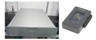
Figure 2: LLRF control system (Left) and Myrio 1900 (Right).
