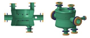
Figure 1: Geometry of the SPS DQW crab cavity.
