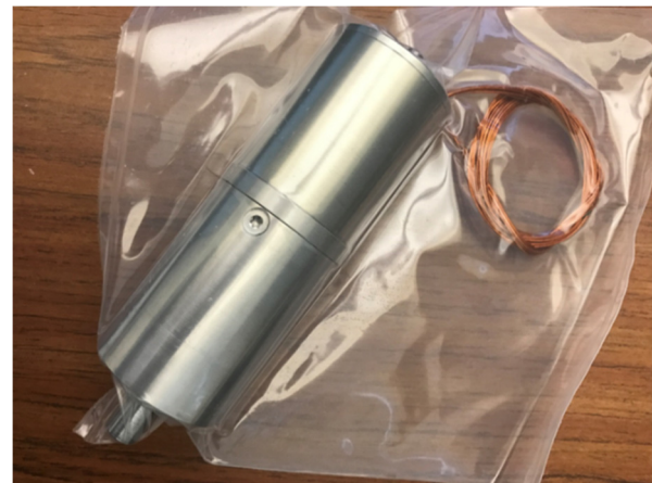
Figure 5: Photograph of the Phytron cryogenic stepper-motor with 1:100 harmonic drive gearbox.
