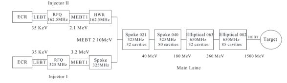
Figure 1: Schematic layout of the C-ADS driver linac.
