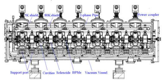
Figure 3: Longitudinal section of the cryomodule.
