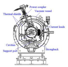
Figure 2: Transverse section of the cryomodule.
