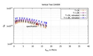
Figure 6: Results of the vertical cryo test of "Cavity 009". Break down at 16.7 MV/m without Field emission.
