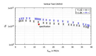
Figure 4: Results of the vertical cryo test of "Cavity 010".  $Q_0 = 1.6 \cdot 10^{10}$  at 12.5 MeV and 2 K was reached.
