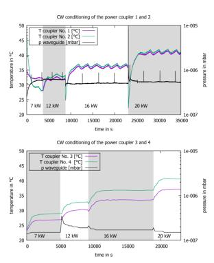
Figure 7: Conditioning of the four couplers at HZDR. A stable operation at 20 kW was achieved.
