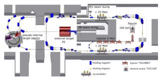
Figure 1: Current design of the MESA lattice. The accelerator is centred around the external beam (EB) mode beam dump. The fixed target experiment P2 is located in the accelerator hall, while the pseudo-internal target MAGIX is located in a separated hall.
