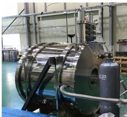
Figure 11: Photograph of the High Tc superconducting quadrupole prototype.
