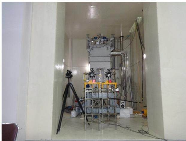
Figure 5: Photograph of the assembled QWR cryomodule in the horizontal test bunker.
