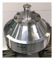
Figure 3: Picture of mushroom-shaped Aluminum cavity.
