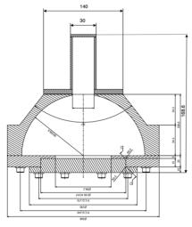
Figure 2: Cross-sectional drawing of mushroom-shaped Aluminum test cavity.
