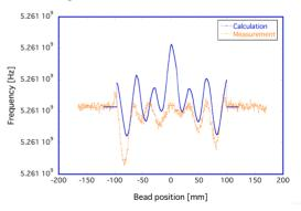
Figure 5: Comparison of bead-pull frequency shift between bead-pull measurement (orange) and CST calculation (blue), at 5.261GHz mode.
