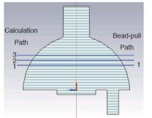
Figure 4: Paths of Bead-pull measurement (right side) and frequency shift calculations (left side).
