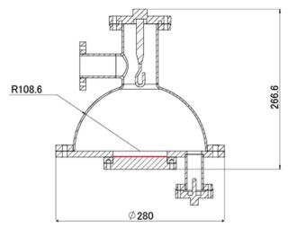
Figure 7: Cross-sectional drawing of mushroom-shaped Nb cavity. (Red line shows sample surface.)
