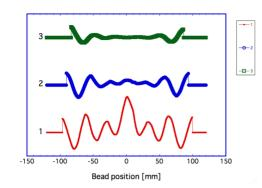
Figure 6: Comparison of calculated frequency shift on the three paths at 5.261GHz mode.
