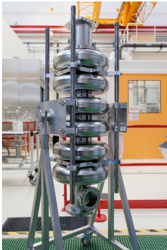
Figure 2: Medium beta cavity.
