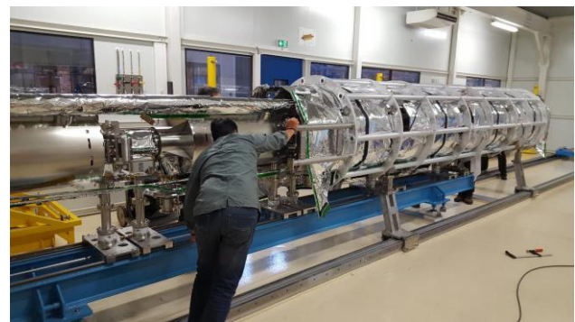
Figure 8: Cavity string insertion in the spaceframe.
