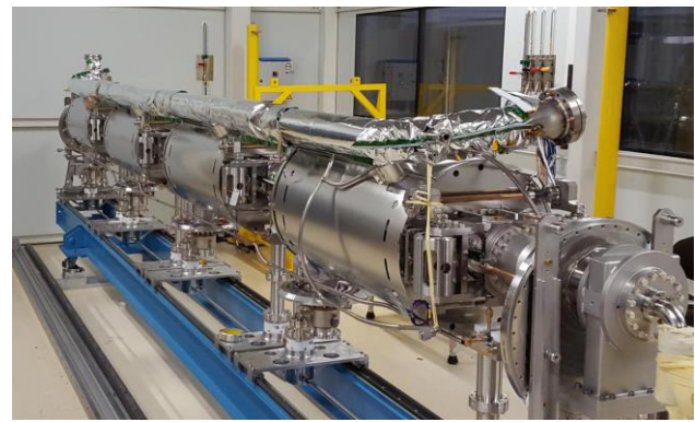
Figure 7: Cavity string dressing outside clean room.
