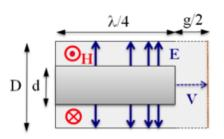
Figure 1: Quarter Wave Resonator (QWR).
