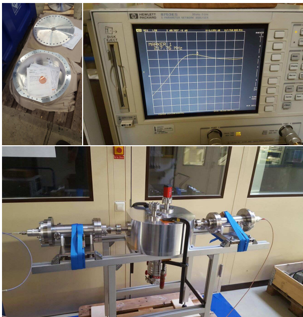
Figure 9: From top left to bottom: Single components, first measurement and picture of the assembly with two FPCs of the newly developed test bench.
