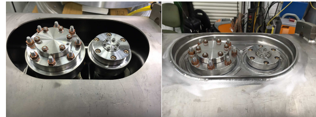
Figure 2: Left: Separated helium vessel (cut out profile including membrane bellows). Right: Replacement trough welded into the helium vessel.
