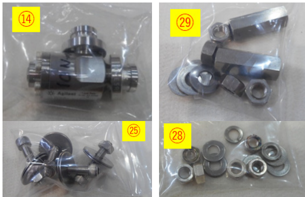
Figure 3: Picture of highly magnetized components. Number in the pictures are reference for Table. 1.
