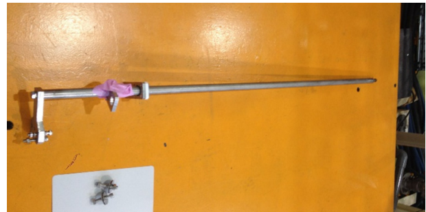
Figure 4: Highly magnetized SUS304 shaft, which is for variable input coupler.
