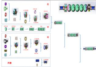
Figure 5: The fabrication process of 5-cell cavity.
