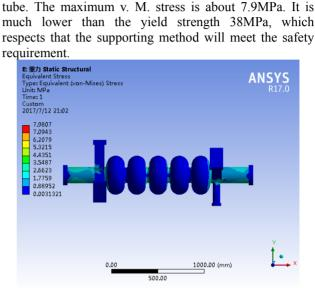
Figure 3: v. M. Stress distribution under self-gravity.
