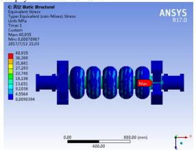
Figure 4: v. M. Stress distribution when inside of the cavity is vacuum.
