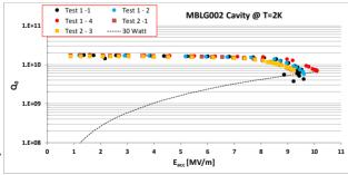
Figure 11: MBLG002 four power rises together with the equi-power line at 30 W.
