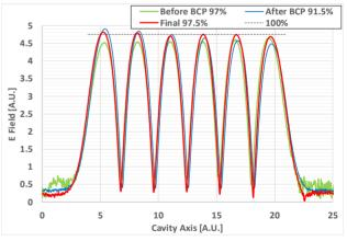
Figure 6: MB001 cavity field profile evolution before and after "Bulk BCP" and after final tuning.
