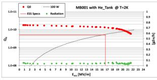
Figure 10: Performances of MB001 integrated in the He-Tank.
