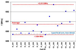
Figure 3: HC frequency distribution. The dotted light blue line is the simulated frequency value from Superfish, keeping into account the cell extra metals at iris and equator.
