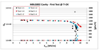
Figure 12: MBLG002 Q<sub>0</sub> vs Eacc plots showing FE.
