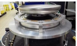
Figure 2: Installation of a dumb bell on the set up for RF check.
