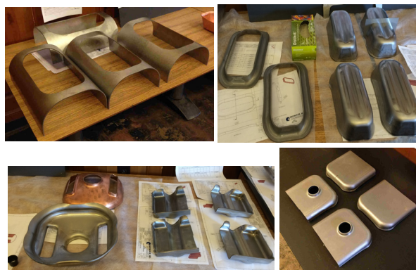
Figure 2: Formed parts of the two rf-dipole cavities.
