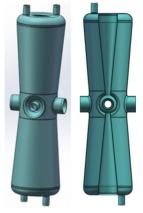
Figure 1: The 162.5 MHz, high current  $\beta$ =0.09 HWR cavity designed by Peking University.
