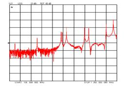
Figure 7: HOM spectrum of the HWR cavity.
