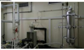
Figure 4: BCP treatment of the HWR cavity.
