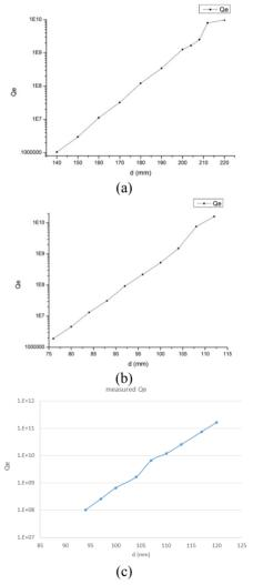
Figure 9: Qe v.s. position of the test antenna tip. (a) Simulation result of Qe calculation when power feeds in from the coupler port. (b) Simulation result of Qe calculation when power feeds in from the beam pipe port. (c) Measured result of Qe when power feeds in from the beam pipe port.
