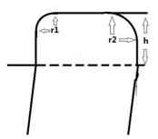
Figure 3: shape of the short plate with different blending radii with the conductors, R1 is the blending radius with the inner conductor and r2 with the outer conductor.
