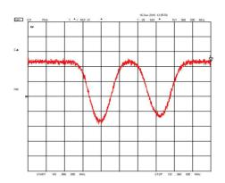
Figure 8: The electric field distribution along the cavity axis.
