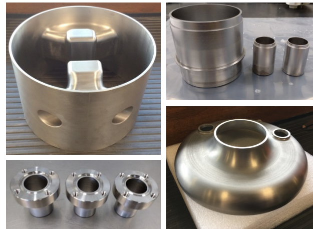
Figure 3: Clockwise from top left: the fully machined centre body, a beam pipe and RF tubes, end cap, and the welded RF port assemblies.
