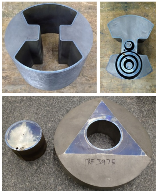
Figure 2: The niobium pieces after EDM. Clockwise from top left: The centre body piece, the offcuts, and the end cap piece with offcut.
