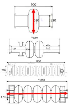
Figure 1: Sketches of four types of cavity prototypes which may need EP at IHEP. The frequencies of cavities from upper to lower are 500MHz, 650MHz, 1.3GHz, and 650MHz, respectively.
