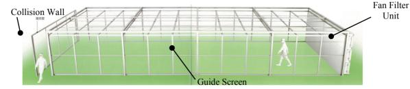
Figure 2: Floor KOACH Ez, source of drawing: product catalogue of KOKEN LTD...
