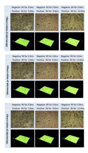
Figure7: Surfaces after BP-EP process for 10 minutes each with changing the condition of pulse-shape.
