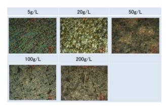
Figure5: Comparison of surfaces after PB-EP process with NaCl electrolyte at the concentrations of 5, 20, 50, 100, and 200 g/L.
