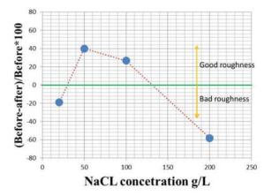
Figure 6: Comparison of the surface roughness of Nbcoupon samples by BP-EP processes with various concentrations of NaCl electrolyte.
