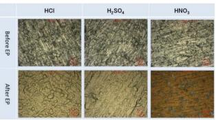
Figure 3: Observation of surfaces before and after BP-EP processes for HCl, H<sub>2</sub>SO<sub>4</sub> and HNO<sub>3</sub> solutions.
