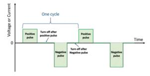
Figure 1: Typical wave form of periodic Bipolar-Pulse (BP) current.
