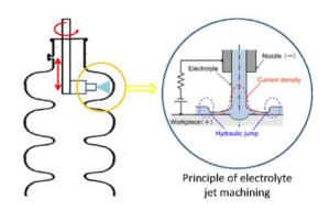
Figure 8: Application of electrolyte jet machining to SRF Nb cavity.
