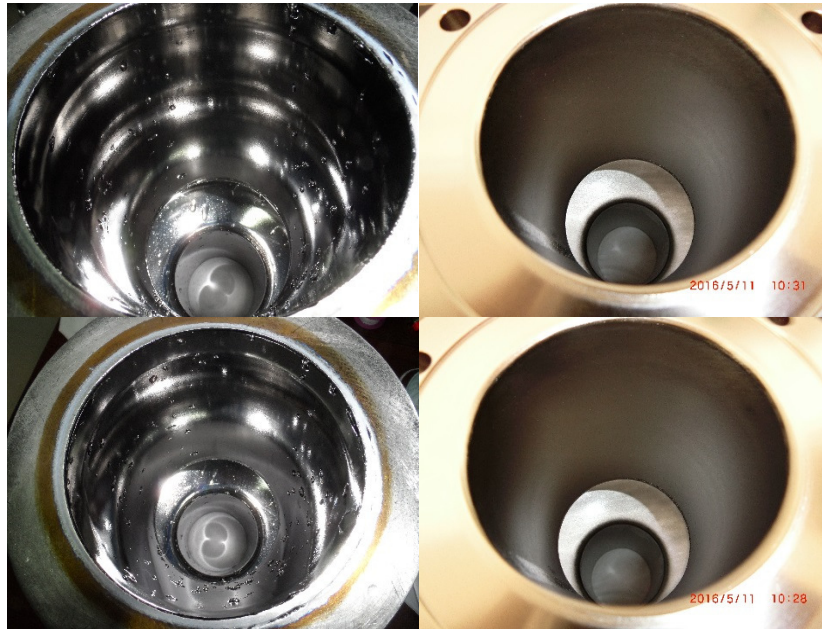
Figure 5: The inner surface of one-cell cavities after EP (left) and BCP (right).
