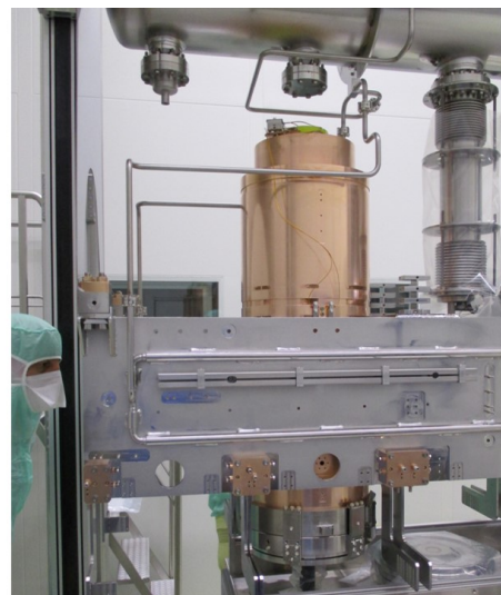
Figure 10: Test blank assembly on the CM.
