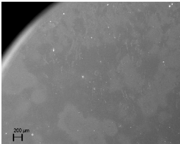
Figure 3: SEM image of a Nb-Pb photocathode with 2 μm Pb film with spherical extrusions.
