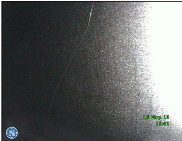
Figure 4: Scratch along the inner conductor observed after the first Dewar test ( \beta = 0.085 QWR, S85-952).
