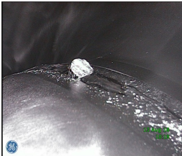
Figure 5: Electron-beam weld repair of inner conductor to short plate blow-through with plug not fully melted, observed during incoming inspection ( \beta = 0.53 HWR, S53-125).
