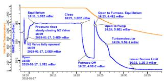
Figure 2: Temperature of the furnace and vacuum pressure of the hot-pot during bake-out of samples in a 100 mbar nitrogen atmosphere.
