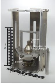
Figure 3: Newly designed variable input coupler for VTC  $Q_0$  and E measurements with minimal uncertainties. The coupler is mounted on top of the cavity, allowing variation of  $Q_{ex}$  during measurement. The input antenna is shown right of the coupler. The coupler is build from steel 1.4429 and aluminium.
