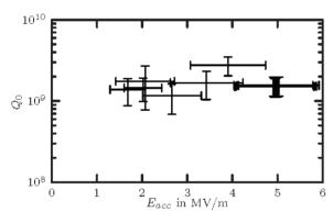
Figure 8: Measured Q vs. E values of a single cell cavity. By reasons of erroneous rf equipment the uncertainties are large and the results will be corrected in a repeated measurement.
