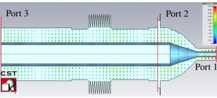
Figure 5: Cross section view of the CST MWS simulation of the variable input coupler for the vertical bath cryostat. The scattering matrix components have been calculated for different port combinations. The port locations are indicated by the red lines.
