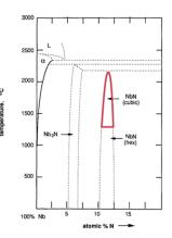
Figure 1: Nb-N binary phase diagram. The cubic  $\delta$ -NbN, on which the research at the S-DALINAC is concentrated is highlighted. It forms at temperatures above 1300°C [8].
