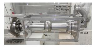
Figure 6: Photograph showing a 3 GHz single cell cavity in the VT assembly. The input coupler is mounted on the left side (top in VT) of the cavity. The as well new designed output coupler is mounted on the right side (bottom in VT) of the cavity.
