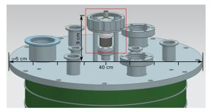
Figure 4: Highlighted is the nut assembly in the center of the VT closure which allows changing of  $Q_{ex}$  during measurement runs.
