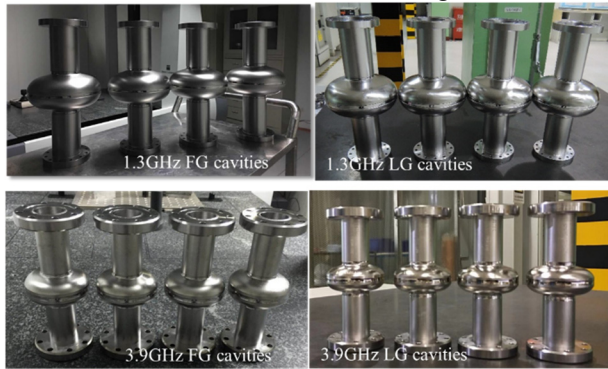
Figure 1: 16 single-cell cavities made in FG and LG Nb.
