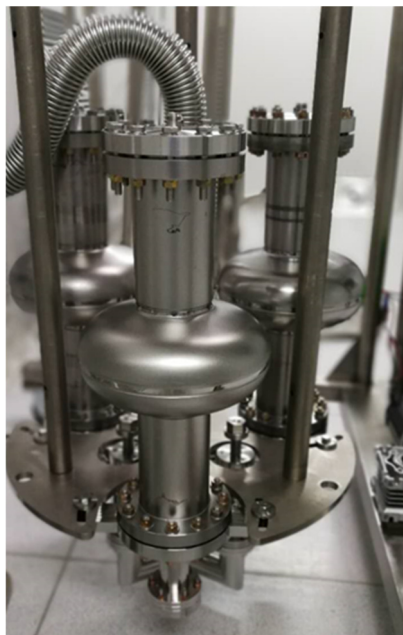
Figure 3: Single-cell cavities cleanly assembled on the insert for vertical test.
