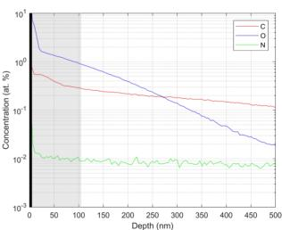
Figure 4: SIMS measurement of atomic concentration of impurities in a witness sample baked with cavity SC-06 in its infusion run. Black bar indicates surface oxide; gray bar approximates RF penetration layer.
