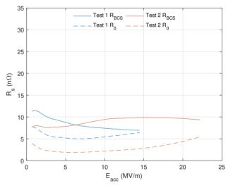
Figure 7: RF test results of the two infusion tests of cavity LTE1-1. R<sub>BCS</sub> taken at 2 K. Peak field shown here does not indicate quench field.
