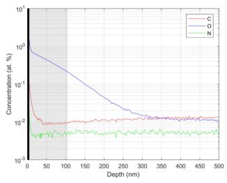
Figure 8: SIMS measurement of atomic concentration of impurities in a witness sample baked with cavity LTE1-1 in its infusion run. Black bar indicates surface oxide; gray bar approximates RF penetration layer.
