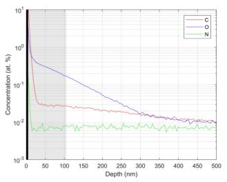
Figure 6: SIMS measurement of atomic concentration of impurities in a witness sample baked with cavity RDTTD-4 in its infusion run. Black bar indicates surface oxide; gray bar approximates RF penetration layer.
