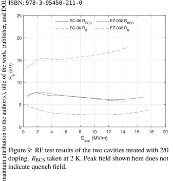
Figure 9: RF test results of the two cavities treated with 2/0 doping. R<sub>BCS</sub> taken at 2 K. Peak field shown here does not indicate quench field.
