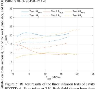
Figure 5: RF test results of the three infusion tests of cavity RDTTD-4. R<sub>BCS</sub> taken at 2 K. Peak field shown here does not indicate quench field.
