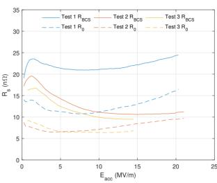
Figure 3: RF test results of the three infusion tests of cavity SC-06.  $R_{BCS}$  taken at 2 K. Peak field shown here does not indicate quench field.
