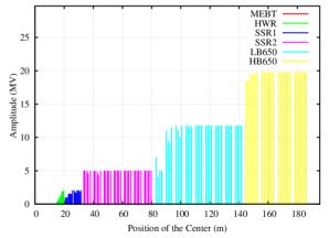
Figure 5: Voltage amplitude settings in cavities along the linac for the baseline optics.
