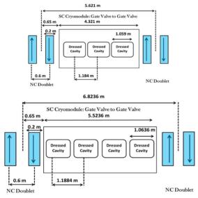
Figure 2: Focusing period in LB650 section for (top) 3cavity and (bottom) 4- cavity cryomodule. Note that, upward and downward arrows depict vertical focusing and defocusing quadrupole respectively.
