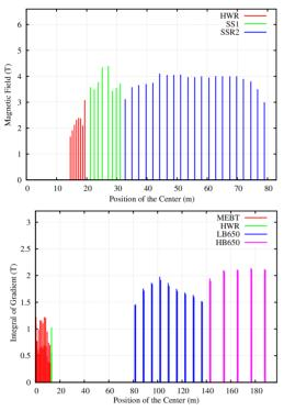
Figure 6: Axial fields (top) and integral fields (bottom) settings in solenoids and quadrupoles respectively for the baseline optics.
