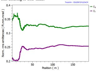
Figure 8: RMS normalized transverse (magenta) and longitudinal (green) emittance along the linac.
