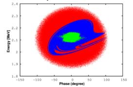
Figure 9: Longitudinal acceptance of the PIP-II SC linac (blue) with  $6\sigma$  beam (green) at the SRF linac entrance. Initial particle distribution was shown in red.
