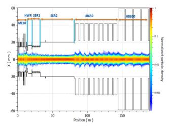
Figure 7: Beam density projection in horizontal plane along with aperture limitation through the RFQ exit to the linac end.
