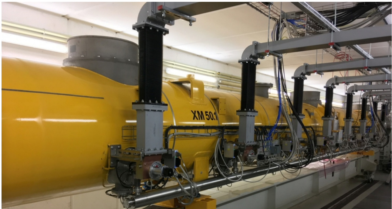
Figure 1: Module XM50.1 on the Module Test Stand XATB2 in AMTF.
