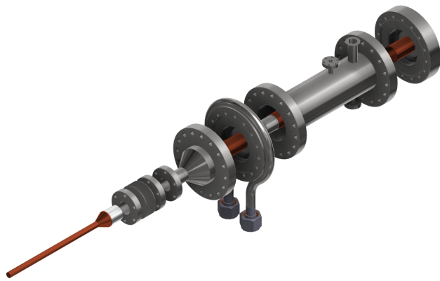
Figure 2: New modular design of the power coupler with two window-flanges.
